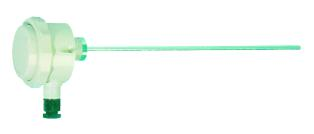
For certain applications involving measuring the temperature of process chemical vessel such as acid etch baths where Stainless steel does not have the necessary chemical resistance, TPA - 2 & TPA- 3 probes can be supplied with 6mm dia. plain bodies P.T.F.E. sheathed.
