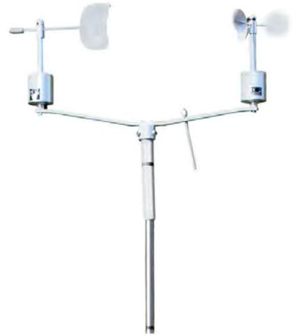
of our new BC7635 slave controllers to display the results in degrees of rotation from north IE North is 0o East is 90o South is 180o some clever electronics allowed the unit to ignore buffeting of the wind. The recorder and indicator were built into a GRP control panel for quick and easy site installation. When the panel had been
